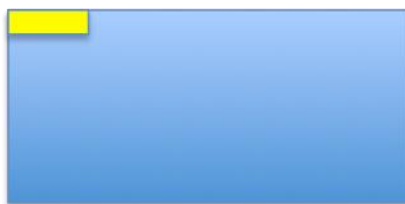
Figure 6.2: Comparison of ground pixel sizes. Nadir pixel as yellow square (30km x 60 km), limb pixel as blue area (400km x 240 km) that results into a tropospheric pixel of 60km x 240km.
