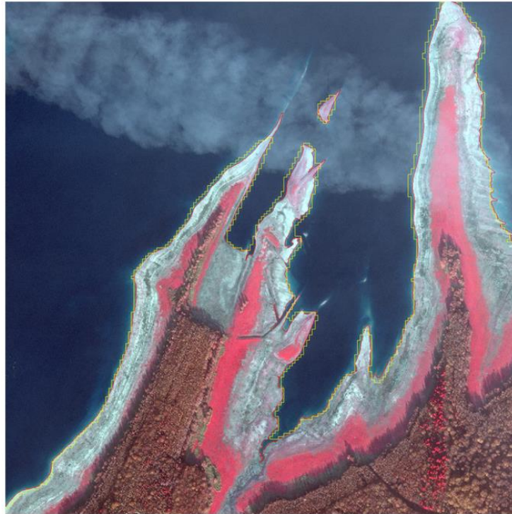
Figure 3 Comparison between Sentinel2 and a Pleiades NEO water extent limit, respectively in yellow and red; the overall accuracy is 98,82%.
