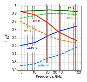
Figure 2-11: NORSEX radiometric signatures
