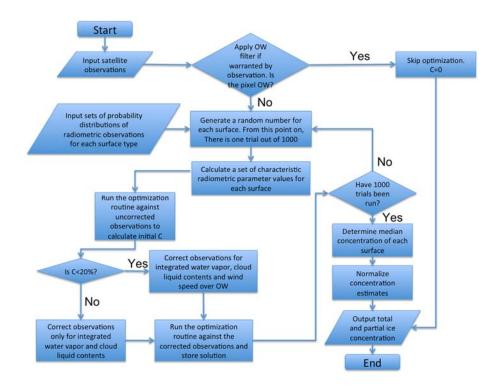
Figure 5-9: Flowchart of the ECICE algorithm
