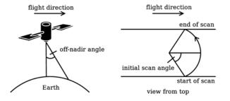
Figure 2-14: Viewing geometry of AMSR-E (Wiebe et al. 2008).
