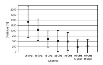
Figure 2-16: Residual, random geolocation error after geolocation correction (Wiebe et al. 2008).
