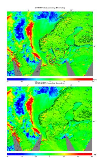
Figure 2-15: AMSR-E 89 GHz B-Scan ascending – descending brightness temperature differences. Left: original (JAXA) geolocation. Right: UB geolocation.
